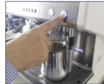
Purge Steam Wand
