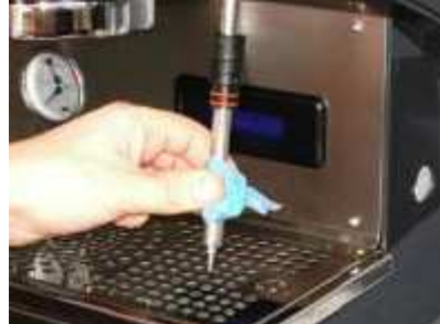
Clean the GTV nozzle with a sponge moistened with detergent for milk. (ref 1011011)
