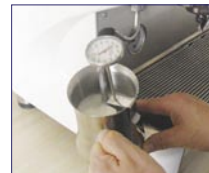
Tip of Steam Arm Just Below Surface of Milk
